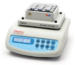
The Thermo Scientific Thermal Mixer offers variable speed and temperature control with a choice of blocks for microtubes and microplates.
